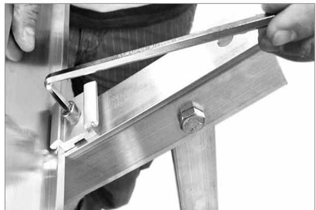
Tightening the upper clamps
